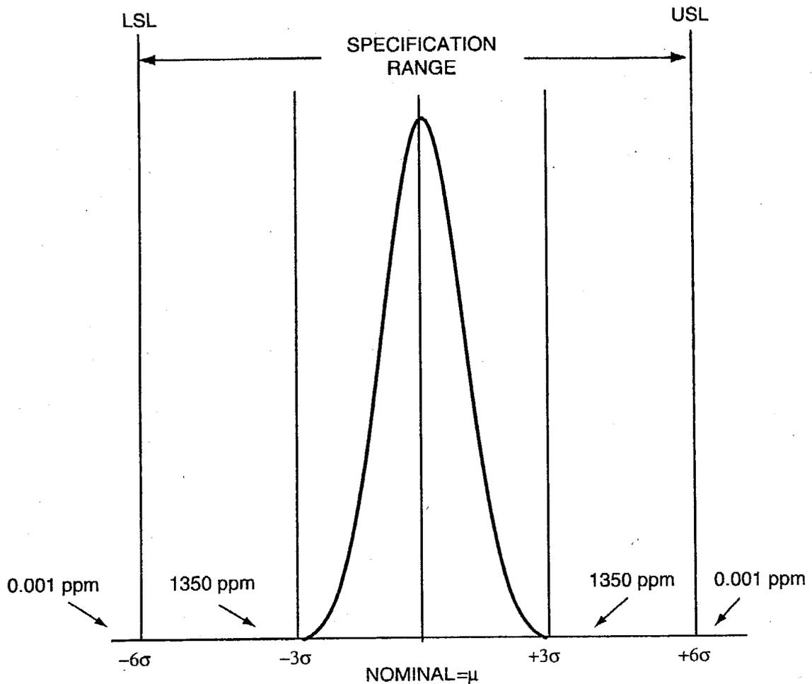
**Figure 1.** A normal distribution showing “defective” parts per million (ppm) at the three and six sigma levels (Pyzdek, 1999, p. 141).
